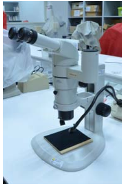
Figure 8. Nikon SMZ800 Stereomicroscope used during analysis
