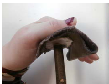
Figure 24. The use of shell and leather to protect the hand at the top of the drilling shaft
